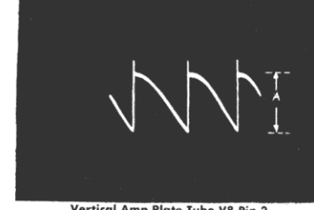
Vertical Amp Plate Tube V8 Pin 2 Sweep Non-Linear Due to Extreme Position of Control A=125 volts
