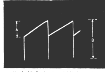
Vertical Deflection Amp Grid Tube V8 Pin 4 A=60 volts B=85 volts
